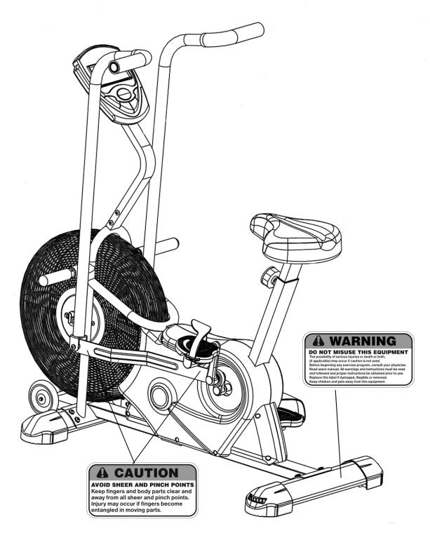
The Warning Labels and Caution Label shown here have been placed on the Rear Stabilizer, Main Frame. If the labels are missing or illegible, please call customer service at 1-800-999-8899 for replacement. Apply the labels in location shown.
